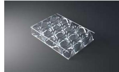
The distinctive TRCore for our clear-PEP<sup>®</sup> panels is manufactured on our specially designed and patented core expander. The innovative characteristic of the special cell structure gives the lightweight panels not just a unique depth but also an extremely high rigidity.
